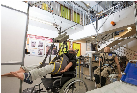
MARIONET-ASSIST, cable parallel robot for the assistance of persons with reduced mobility
