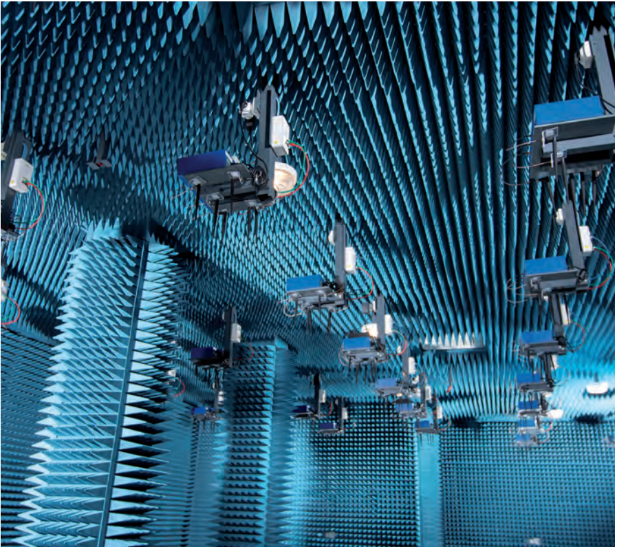
Anechoic room of the FIT (Future Internet of Things) experimental platform. © Inria / Photo C. Morel.
